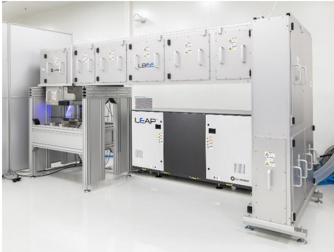
Image 2: A new excimer laser system is now available at Fraunhofer ILT for process development in surface microprocessing. © Coherent, Inc.
