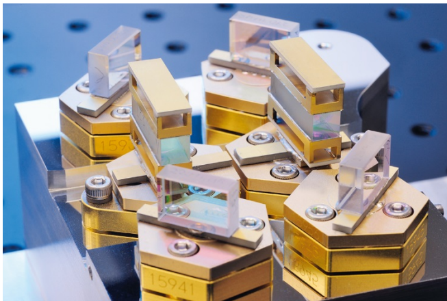
Image 2: Optical parametric oscillator (OPO) for the MERLIN-LIDAR system, based on FULAS, the new Future Laser System from Fraunhofer ILT. © Fraunhofer ILT, Aachen, Germany.
