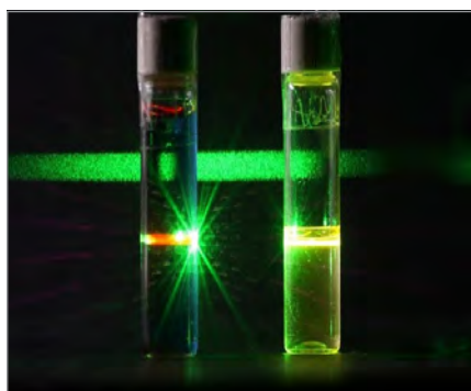
Green fluorescence of a dye solution excited with blue light
