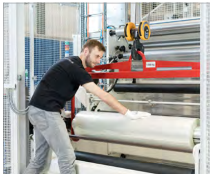
1.25 meter wide film substrate on the roll-to-roll coating line atmoFlex 1250
