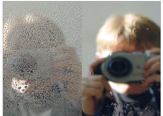
Superhydrophilic titanium dioxide layer (right) as an easy-to-clean coating
