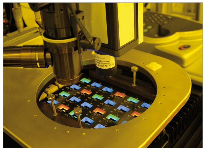
Probe station with patterned OLEDs in the clean room of Fraunhofer FEP
