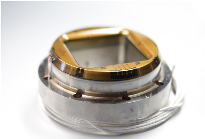
Deep-drawing die with complete sensor system.
