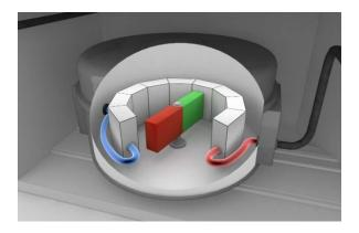
Setup of a magnetocaloric cooling system: The segments shown in gray contain the magnetocaloric material. This material is alternately heated and cooled by the rotating magnet. Because of the internal structure of the segments, heat is transferred to the ambient air on the right side while on the left heat is removed from the container to be cooled. © Fraunhofer IPM
