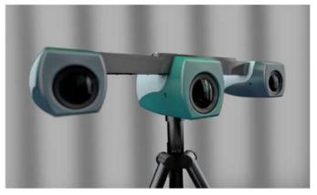
3D sensor technology: two high-speed cameras and a gobo projector capture the 3D data of the moving person.
