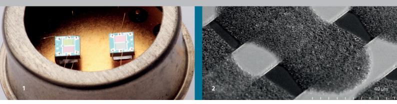
Metal oxide gas sensor array with four different sensitive elements.
