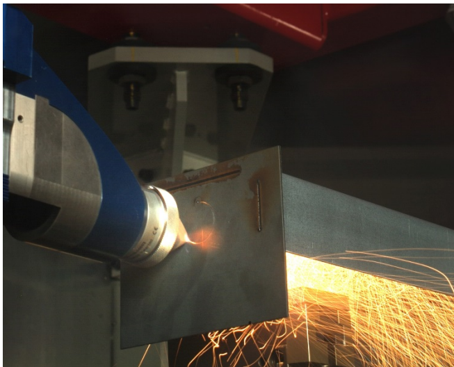
Image 1: A multifunctional laser processing head plays a major role in the new NRW project MultiPROmobil; it enables innovative sheet metal assemblies through the integrated cutting, welding and manufacture of structures additively. © Fraunhofer ILT, Aachen, Germany.
